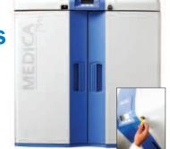
pre-treatment, reverse osmosis, 254 nm UV lamp and ultra micro filtration to produce CLSI Type II pure water that meets and exceeds ASTM D1193, ISO 3696 plus European, USA and Japanese Pharmacopeia standards with guaranteed bacterial specifications <1cfu/mL.
