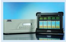
The KARL STORZ OR1 mini is an affordable and simple routing system consisting of a 10.5" tablet and a video image processor, which makes it possible to route different digital and analog signals in the OR.
