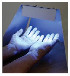
easy to transport. Its electronic power supply means it can be used anywhere in the world. The UV LEDs estimated operating life is 16,000 hours.
